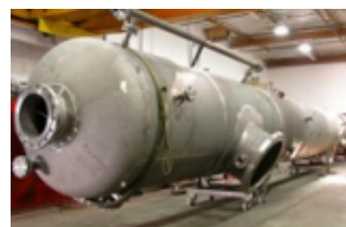
Titan Metal Fabricators titanium column for biodiesel production
