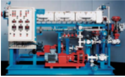
SGL Carbon skid for dilution of sulfuric acid
