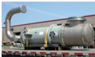
Titan Metal Fabricators titanium thermo-syphon reboiler for biodiesel production
